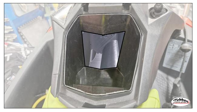
12. Use the holes in the glove box extension as a guide and drill through the storage box using a Ø4,5mm Drill Bit (#16)
