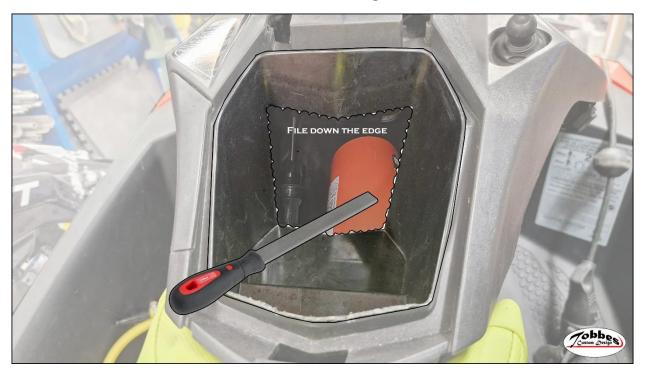
9. Then mount the box and check that the edges are flush with the box
