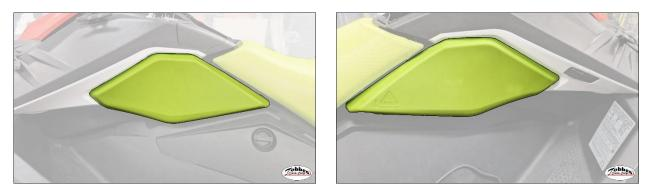
2. Use a trim pin remover and 8mm driver to remove both trim panels above knee panels to better access
