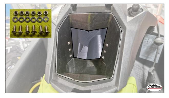
14. Wipe off any excess glue and feel to make sure there are no sharp edges
