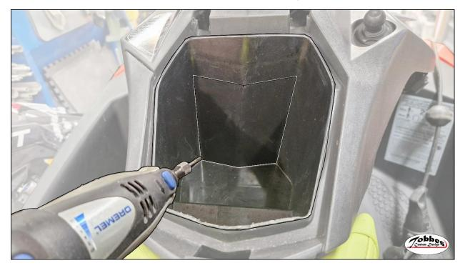
6. Drill small holes with a \$\vec{\vec{\vec{9}}}\_5-8mm drill bit on the inside and along the entire line
