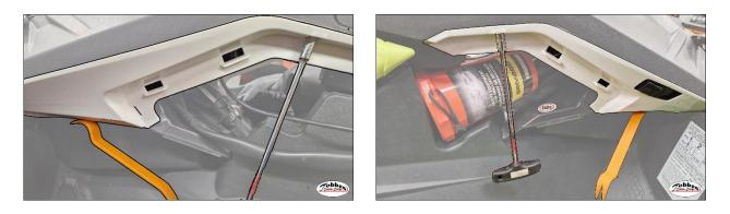
3. Check the fit of the Glove box extension
