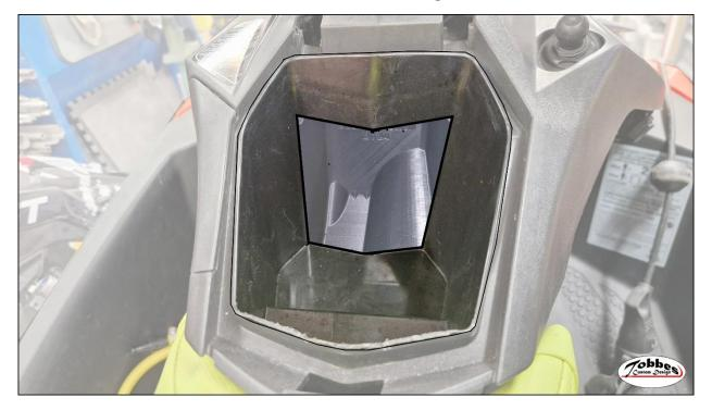
10. Remove the extension, apply silicone around the rim of the glove box extension before reinstalling, and wipe off any excess.
