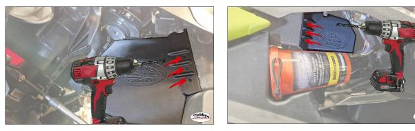
13. Complete the installation by using 6pc M4x20 with washer and locking nut. Add some silicone on top of the screws for a water-tight seal.
